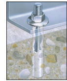
Fastening to Concrete with Threaded Rod
